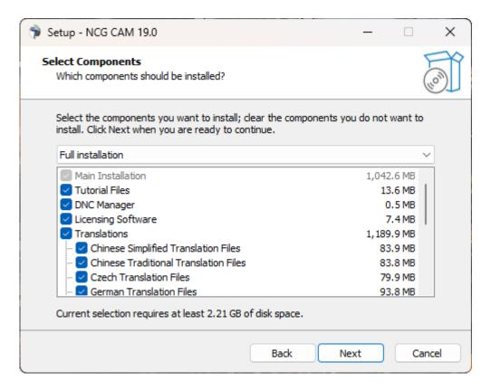
In any case, make sure that the **Licensing software** option is activated. Otherwise you cannot enter a license code for the dongle.
